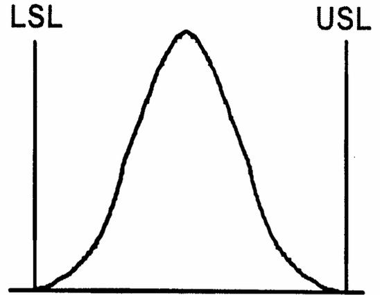
Frequency Distribution showing a Process Capability ( $C_p$ ) of 1
