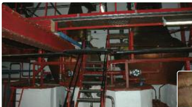
Left: Wash and spirit stills. The inset shows the 'steam kettles' in wash still.
